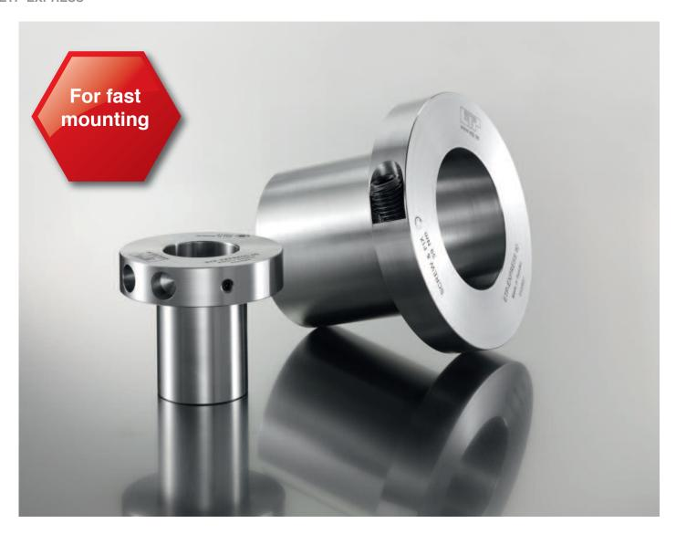
ETP-EXPRESS is available as standard for shafts 15-100 mm, also imperial. Runout ≤ 0,02 mm. Number of mountings 500 - 2 000 (size dependent). The extremely thin built-in dimensions allows for a compact design with low weight and inertia.
