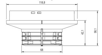
Fig. 2 Dimensioned drawing SCD 563
