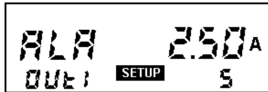
FIG 46 - Selection of the alarm threshold associated with the current of line 1 (number 5)
