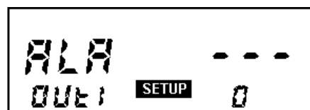
FIG 45 - Setting of alarm on OUT1 output
