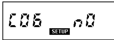
FIG 39 - Disabling the Cogeneration function
