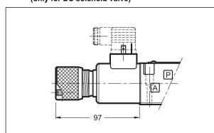
When the set screw is screwed and its point is aligned with the edge of the knob, tighten the knob till it touches the spool: in this position the override is not engaged and the valve is de-energized. After adjusting the override, tighten the set screw in order to avoid the knob loosing.
