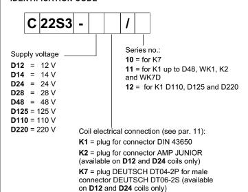
For W7 version only (D12 and D24 only) WK1 = plug for connector DIN 43650
