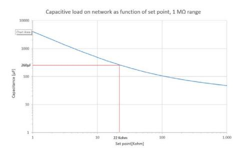
The shown 22 k $\Omega$  set point will accept capacitance up to 260  $\mu F$  on 1 M $\Omega$  range, without false warning.
