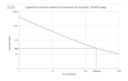
The shown 220 k $\Omega$  set point will accept capacitance up to 26  $\mu F$  on 10 M $\Omega$  range, without false warning.
