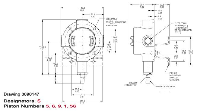
\*Refer to Dimensions table on page 19 for changes in length due to process connection size, including A dimension.
