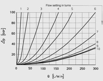
DRV Flow direction from B to A Pressure differential  $\Delta p$  depending on flow rate Q via opened check valve at v = 72 mm<sup>2</sup>/s and t<sub>oil</sub> = 30 °C
