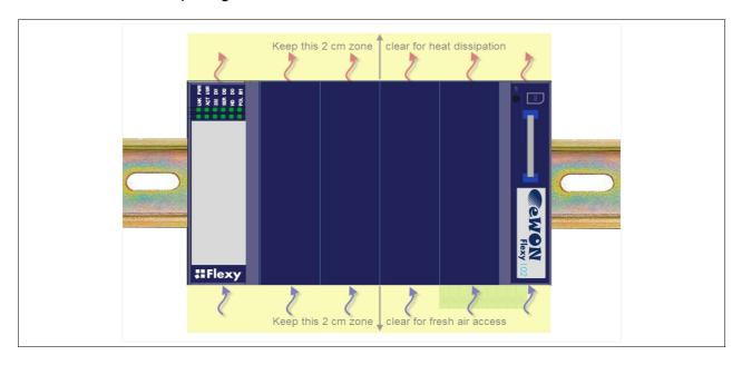
**Caution:** In any other mounting position than the one explained here above, the specified temperature has to be derated to  $-25^{\circ}$ C to  $+40^{\circ}$ C.
