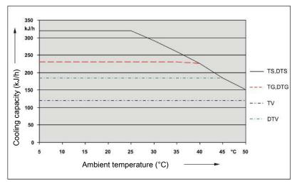
Remark: The limit curves for the heat exchangers exchanger apply to a dew point of 65 °C.
