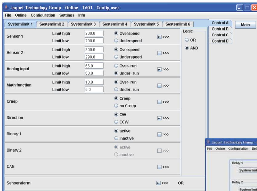
Don't lose time by thinking about parallel- and serial wiring, inverting and double inverting of signals just to get that signal you need. Only think about what signal you finally need and define a System Limit.
